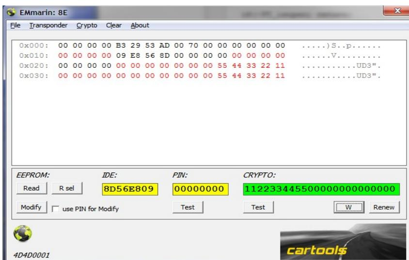
Each EEPROM bank consists of 32 pages, each page means one 16-bit WORD (2 bytes). Wedge type transponders and emulators have only one memory bank (64 bytes total). Remotes have more, typically 8 memory banks. All important data is stored in BANK 0.
