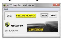
Read or Write emulator: if success, background will change color to green. If no success it goes red (must repeat procedure or verify jumper settings). Emulator must be in configuration mode (both jumpers open).
